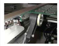
For linear applications the Tru-Trac™ can be mounted above or below the moving object, and the tension on the wheel adjusted for a wide range of applications such as packaging, conveyors, mail sorting, cut to length, labeling, gantries, etc.
